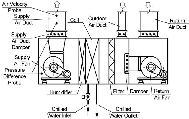
**Figure 8** Measurement points and AHU configuration.
