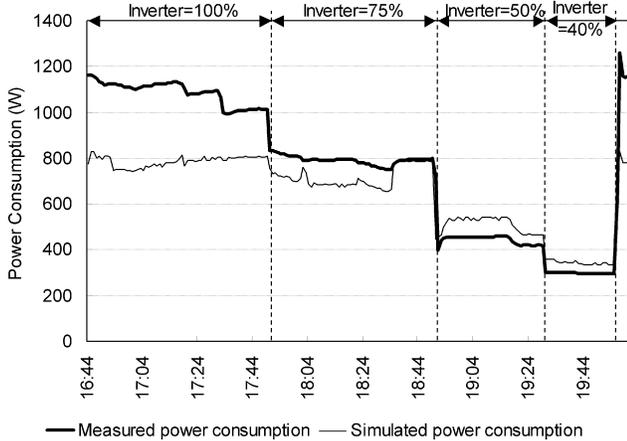
**Figure 11** Total power consumption of a fan subsystem with slipping belts and simulated value with tight belts.
