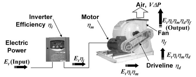
**Figure 3** Components and energy flow of a fan subsystem.
